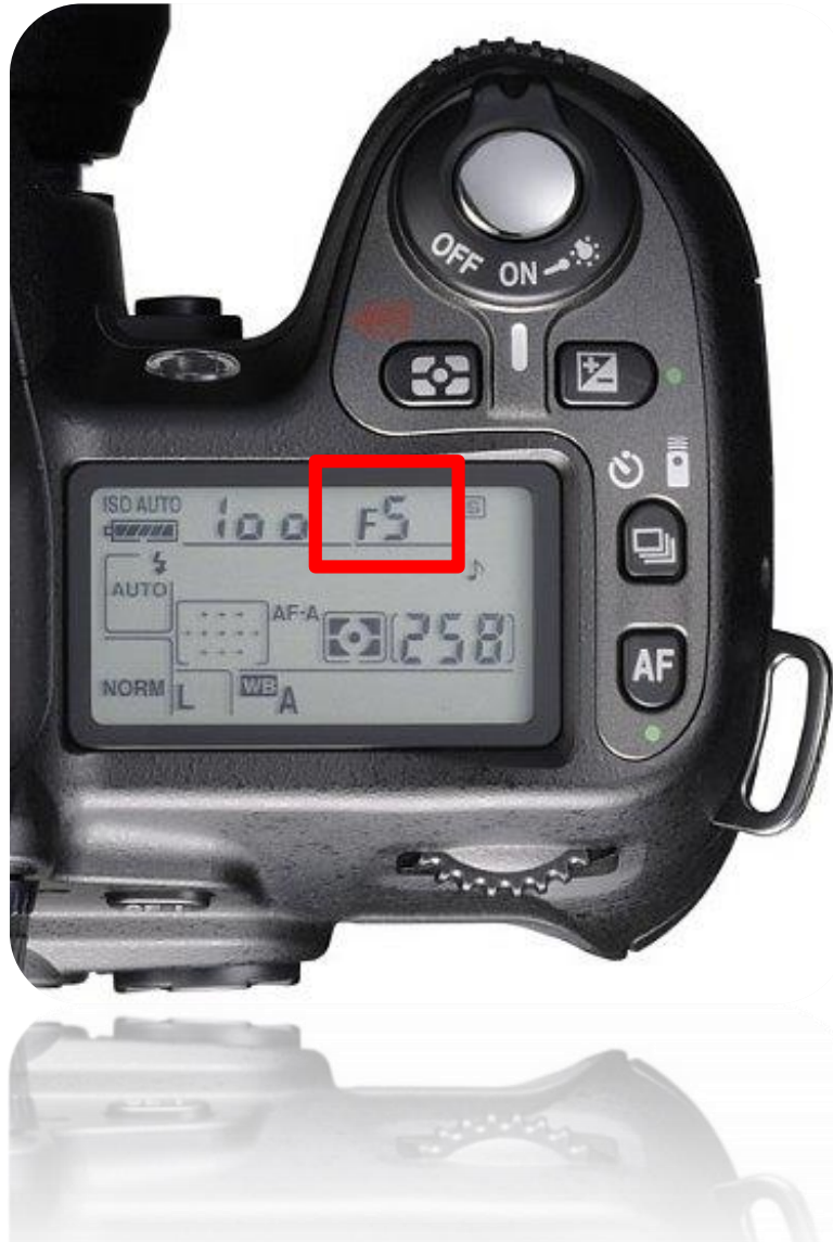
How Apertures appear on the camera
